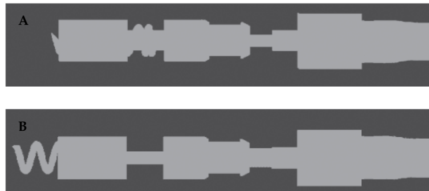
Fig. 7. Rontgen aspect of the unarmed (A) and armed (B) lead's screw (Biotronik original photo)
